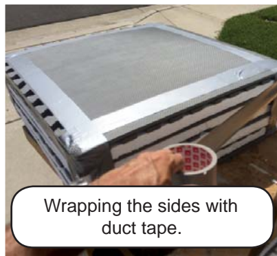
5 layers of styrofoam & 6 layers of floor mat.
