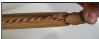
Figure 10: Off-center string indicates a twisted limb.
