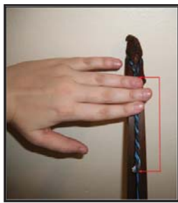
Figure 13: Measuring the twist at the ends of a string.
