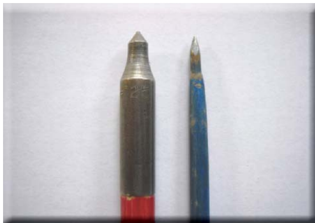
Figure 2: Example of the end of a 3-penny nail placed in a drill hole in the tip of the arrow shaft (shown on the right), replacing the traditional field point (shown on the left) or target tip.
