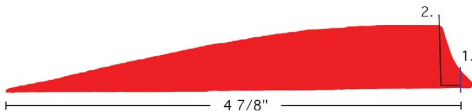
Figure 1: Cutting and measurement diagram for a simple square-end style fletch cut from a shield-cut fletch. Trim the quill to 4 7/8 inches long (1), and trim the barbs into a square shape and trim the excess barbs from the quill at the nock end (2) to create a tab for whipping (the space between 1 and 2).
